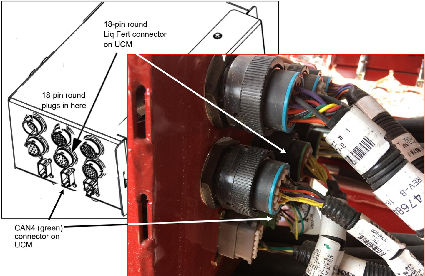
Main Adapter Harness 213-05-3873Y3 plugs into the 18-pin round connector and the 12-pin CAN4 (green) on the UCM on the planter. Unplug the Case connectors in these positions, plug in the SureFire harness, then plug the Case connectors into the SureFire harness. Then plug the Sentinel (or RCM) adapter harness into the ISO and POWER connectors on the 3873 harness.
