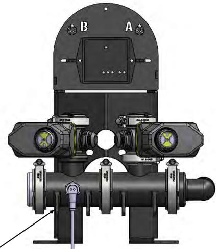
Pressure Sensor for LiquiShift is mounted at the base of the valve stack. The same sensor is used for LiquiShift and displayed on the cab display.
