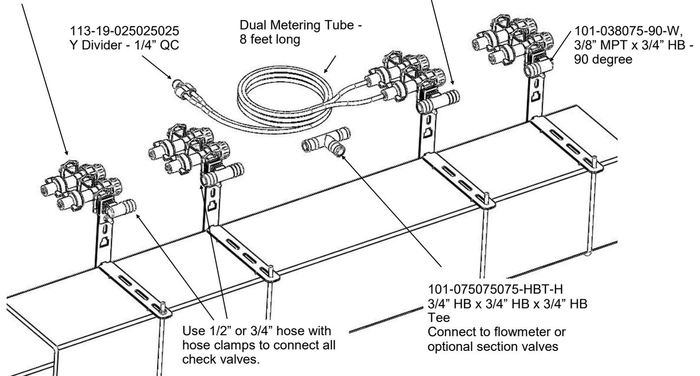
This is a general diagram showing the dual check valve assembly mounted on a planter toolbar. The check valve and bracket are very flexible in their mounting. The check valve can mount behind, directly over, or in front of the toolbar. The check valve can be put in the bracket facing up & down or sideways (shown). In addition, the steel bracket could be rotated 90 degrees and clamp around the bar. The multiple slots in the bracket are used to mount to any tube 7x7 inches or smaller.
