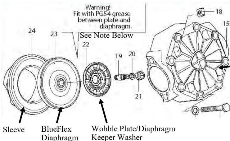
**NOTE: A multipurpose grease is fine to use for applying in between the Diaphragm and Wobble Plate/Washer**
