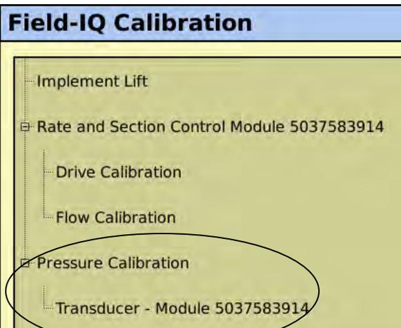
To finish the Pressure Sensor setup, it will be necessary to go to Field-IQ Calibration and select Pressure Calibration and the name of the Pressure sensor you set up.
