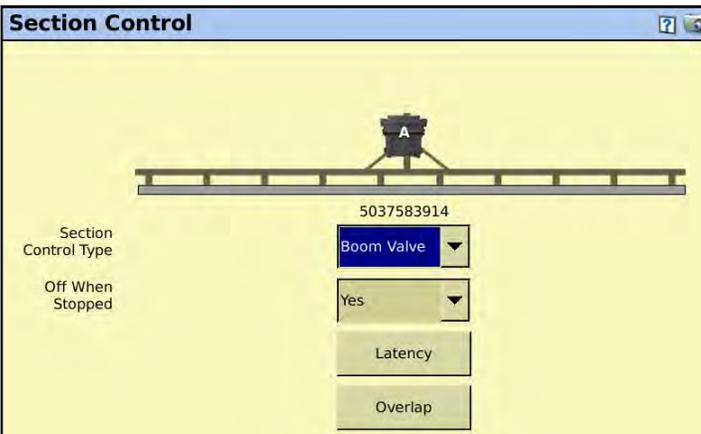
1. Set **Section Control Type** to **Boom Valve**.
