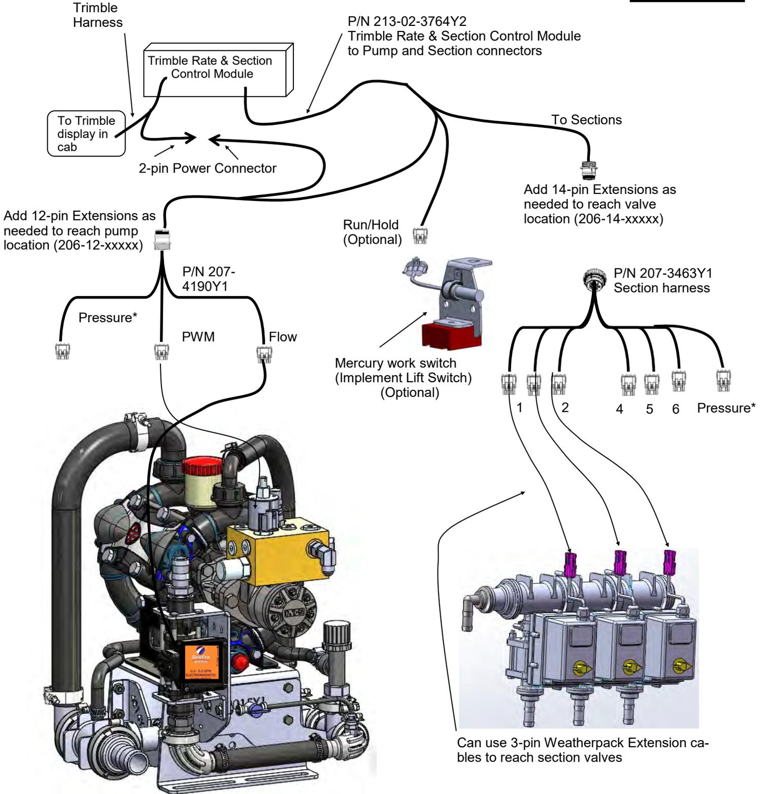
\* The PUMP final harness has a Pressure 1 connector. Section 1-6 has a Pressure 1 connector. Section 7-12 has a Pressure 2 connector.
