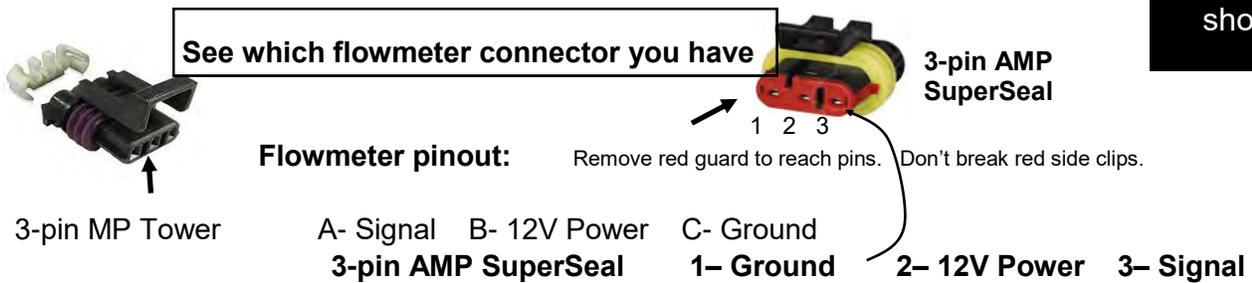
1. Unplug the flowmeter. With voltmeter, check for **12 volts between Power & Ground** of flowmeter connector. Should have **4-5 volts between signal and ground**. If voltage is not present, inspect wiring harness and check for voltage at harness connection(s) nearer the Rate Controller.
