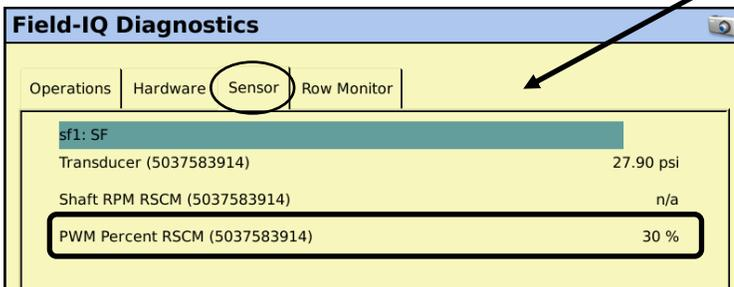
The **Sensor** tab provides information on the Pressure Sensor and Pump Speed (PWM Percent). It is good to know the **PWM Percent** required for normal operation.
