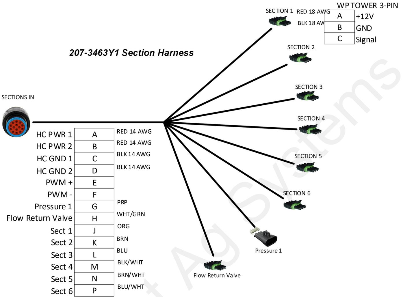
Gen 2 LiquiShift system harness layout—Instead of the section harness shown above (207-3463Y1) connect the following harnessing for the LiquiShift system
