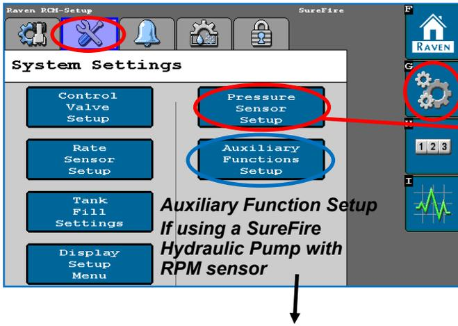
SurePoint recommends putting the Pressure Sensor reading in your **Display Settings** on the Run Screen (see next page). For complete information on how the sensor is operating, go to **Diagnostics > System Information > Pressure Sensors**. 0 Pressure Voltage should be 0.00 V.
