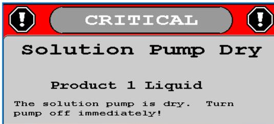
If flow or pressure is not immediately detected, the **Solution Pump Dry** warning will come up and the system will shut down.
