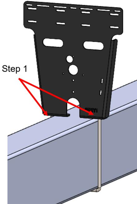
1. Mount 400-4511Y1 to hitch using provided u-bolt.
