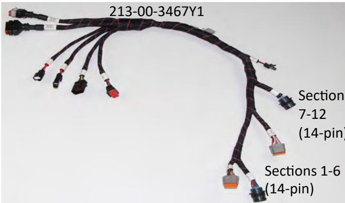
The 14-pin section connector on any SureFire JDRC 2000 Adapter Harness can plug into the LiquiShift 14-pin. With the 3467Y1 harness above, you would plug Section 1-6 connector to the LiquiShift for product 1 LiquiShift. You would plug the Section 7-12 connector to the LiquiShift for product 2 LiquiShift. Product 1 only, product 2 only, or both product 1 & 2 could use LiquiShift.
