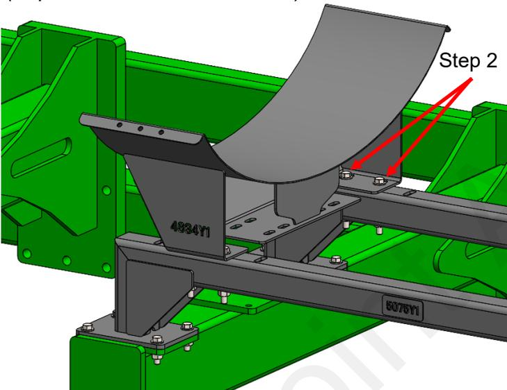
3. Finally, install tank in the saddles and fasten the tank strap mounting brackets, and tank straps. Check for clearance.
