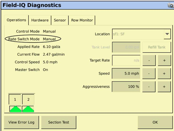
To enable the sections, tap the numbered section tabs above each of the section icons.
