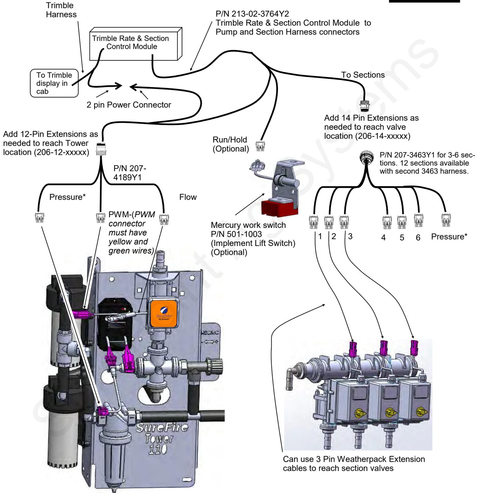
\* It is possible to connect 2 pressure sensors to the Trimble display using the Surepoint xxxxxxY2 harnesses with Pressure 1 and Pressure 2 connections.
