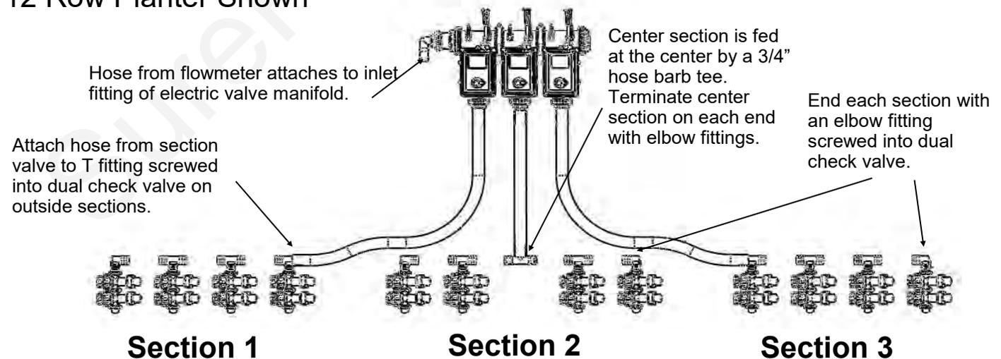
For a **2 section plumbing system**, omit the center section and plumb similar to the outside 2 sections.
