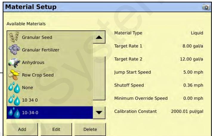
Set **Target Rate 1** & **Target Rate 2** as desired.
