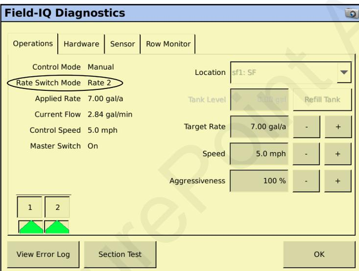
In **Manual** mode, press the + or - button beside Target Rate to increase or decrease the rate.
