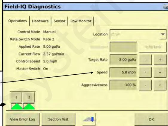
1. Press the + next to Speed to simulate a Speed signal.
