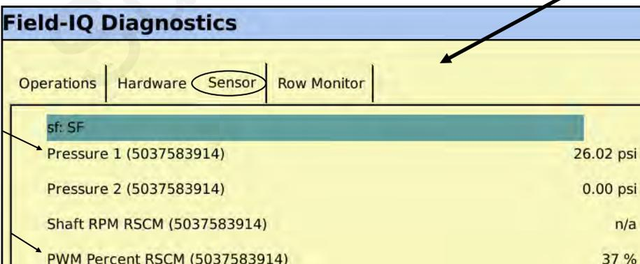
The **Sensor** tab provides information on the Pressure Sensor(s) and Pump Speed (PWM Percent).
