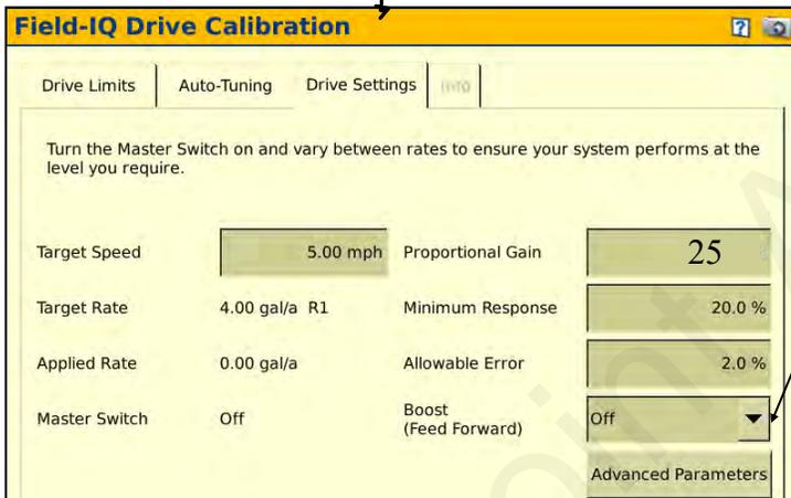
Select the **Advanced Parameters** button to bring up the **Advanced Tuning** screen (shown below). Here you will enter the numbers for the system.
