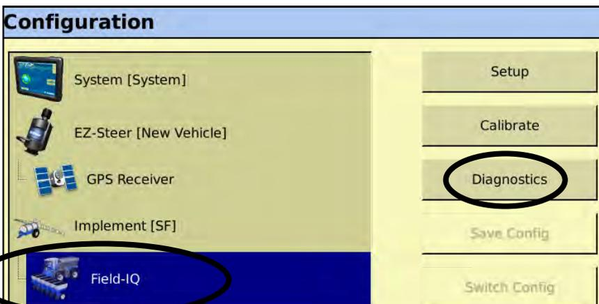
From the Configuration Screen, select **Field-IQ**, then **Diagnostics**. (If the *Diagnostics* tab is grayed out, you probably need to close a Field.)
