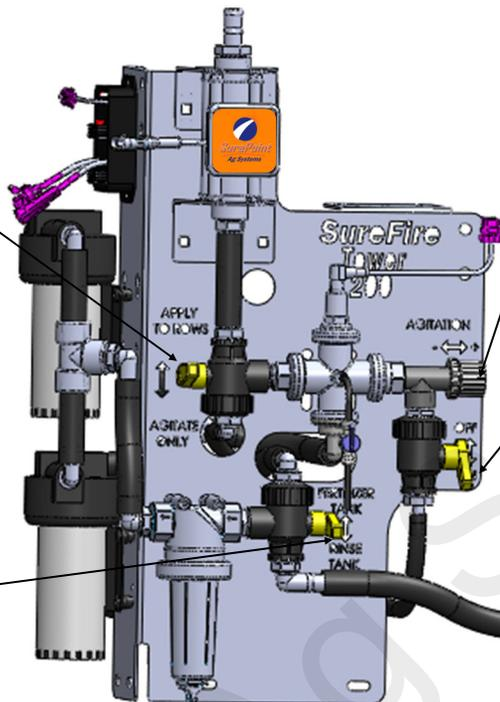
**Agitation Adjust Valve: RECIRCULATION KNOB:** This valve adjusts how much flow returns to the tank while working in the field. Normally closed. If needed, start with a quarter turn.
