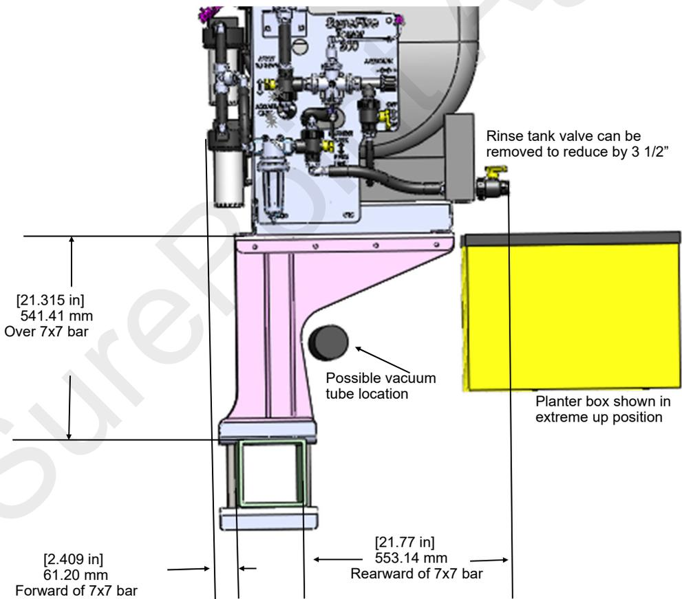
This mount kit includes two welded brackets to mount any of the 3 sizes of accelerator tanks above and offset from the 7x7 planter toolbar as shown.
