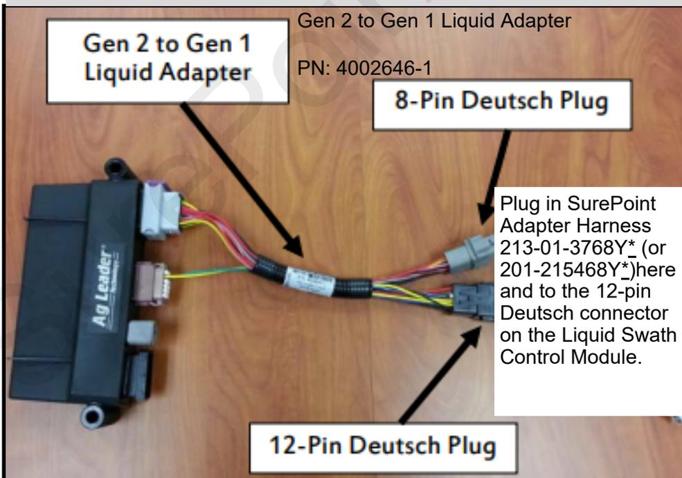
If the ISO Liquid Module is replacing an Ag Leader Liquid Product Control Module, start with the Gen 2 to Gen 1 Adapter and then use the same harnessing that was used before.
