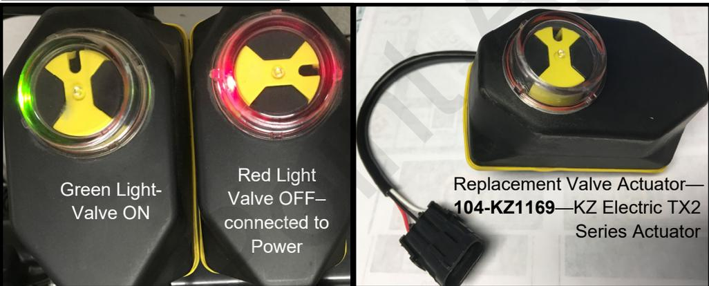
If valve indicator stays GREEN all the time or if valve indicator is not in full ON or full OFF position, replace actuator. Pull gray pin to remove actuator from valve.
