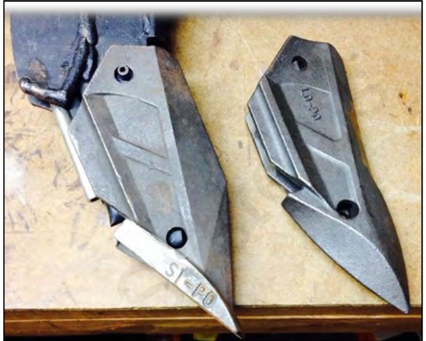
The knife on the left is for no-till conditions. On the right is a less aggressive point for tilled soil.
