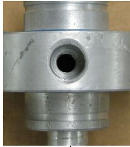
**Threaded orifice not installed**
