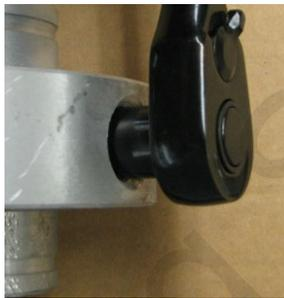
These orifices can be swapped out for different sizes depending on your application needs. Select the correct orifice based on your application needs by referring to the chart below.
