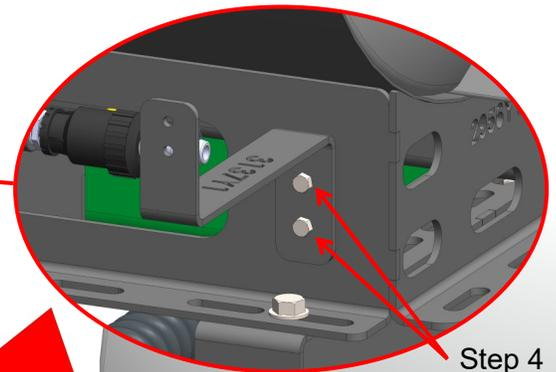
4. Fasten 449-3137Y1 to the tank cradle using two (2) 3/8" x 1" hex head bolts and flange nuts.
