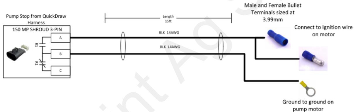
The standard harness is used to break a connection on the motor to make the motor stop. The grounded coil harness is used when the only way to stop the engine is to ground out the ignition coil to stop the sparkplug from firing. On Honda GX370 and GX390 electric start engines, use the following procedure to determine which cable to use.
