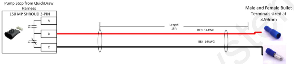
Figure 2: 208-05-2633Y1 Pump Stop Harness (Grounded Coil)
