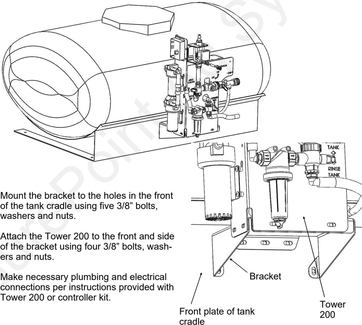
Mount the bracket to the holes in the front of the tank cradle using five 3/8" bolts, washers and nuts.
