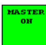
The **MASTER ON/OFF** button enables and disables the Sentinel system. This must be **GREEN (MASTER ON)** for Sentinel to work.
