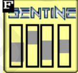
The SENTINEL ROW BAR button appears when using Row Flow Monitoring. If using Rate Control without Row Monitoring, this button will not be used.
