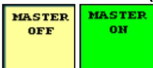
The **MASTER ON/OFF** button enables and disables the Sentinel system. *This must be **GREEN (MASTER ON)** for Sentinel to work.*
