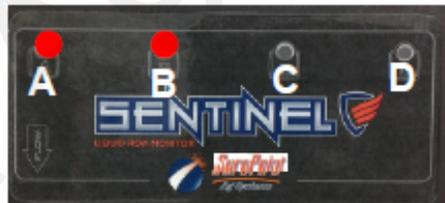
should have lights A & C (1 + 4) come on for 3 seconds when it is plugged in. Unplug the module, watch the lights as you plug it back in.
