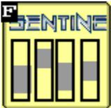
The SENTINEL ROW BAR button appears when using row flow monitoring. When doing row flow monitoring, this takes you to the row bar view page (above). This button may appear on the right side of the screen or on bottom left, where it puts the Row Bar View on the bottom half of the screen.
