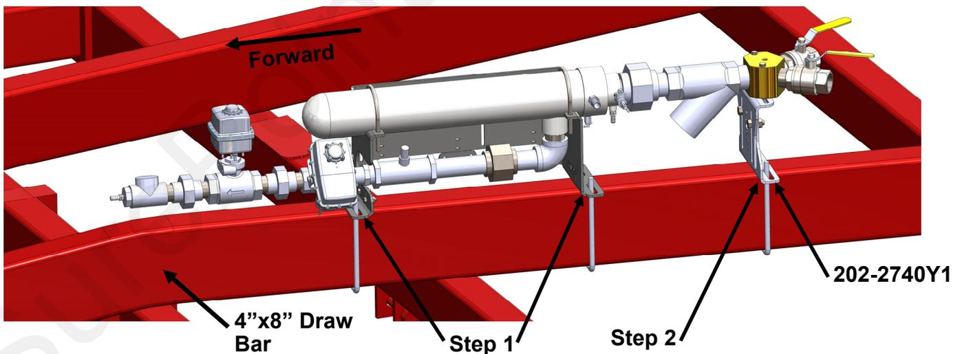
1. Mount the Torpedo to the 4"x8" Draw Bar using the provided 1/2"x4"x9-1/2" Square Bent U-bolts (380-1032). Do not tighten nuts to allow for adjustment in next step.
