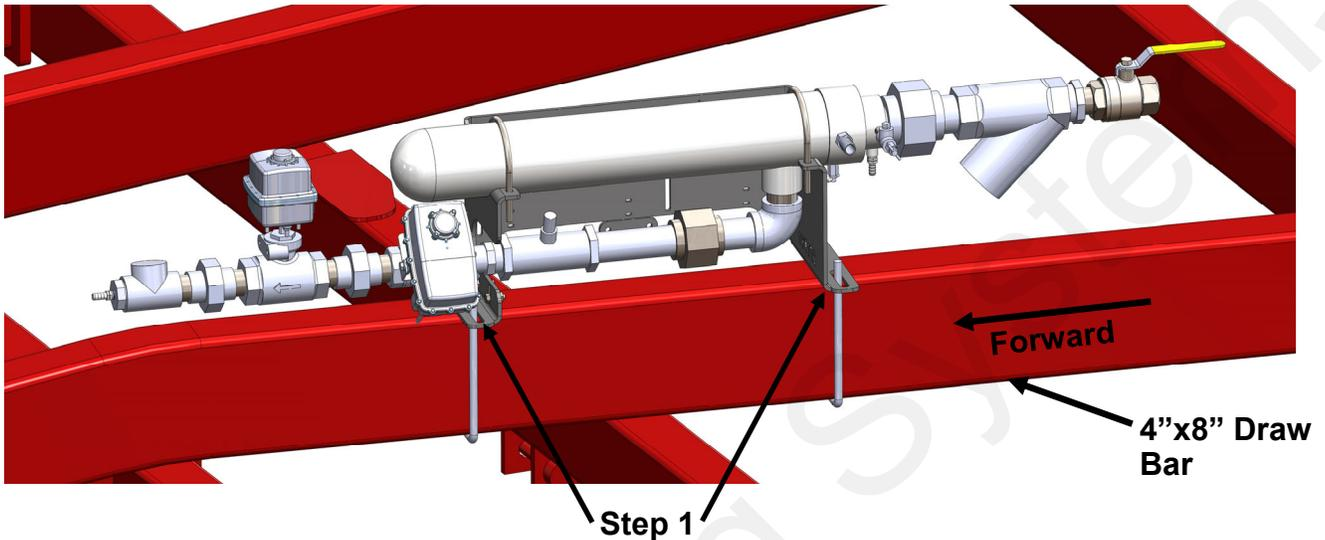
1. Mount the Torpedo to the 4"x8" Draw Bar using the provided 1/2"x4"x9-1/2" Square Bent U-bolts (380-1032). Tighten all nuts once Torpedo is in desired position along the 4'x8" Bar and clearance/interference of existing equipment has been checked.
