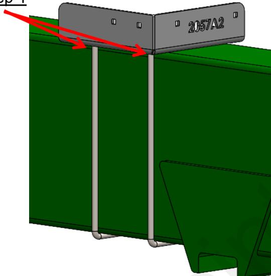
1. Mount 410-2057A2 to the hitch as shown using the U-bolts provided.
