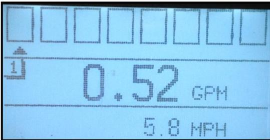
Arrow under Row 1 means the flow in Row 1 is 0.52 GPM.
