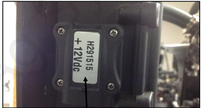
Plug in CAN DEVICE connector here
