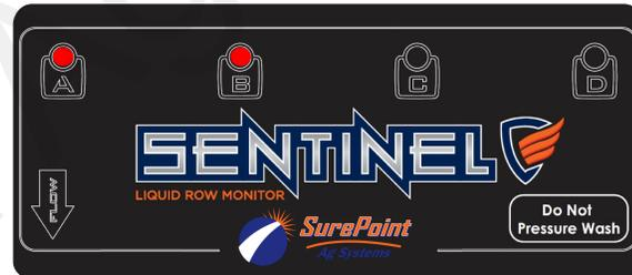
Multiflow Module 4 will show light C when the Sentinel is turned on.
