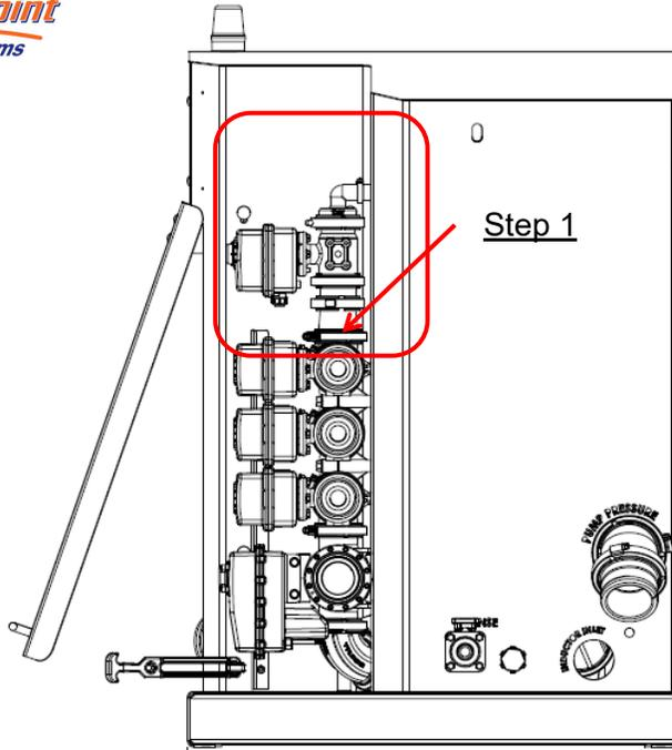
1. Remove clamp/gasket from the top of the 3-way valve manifold, and cut rinse hose. Set the rinse valve assembly aside for re-assembly.
