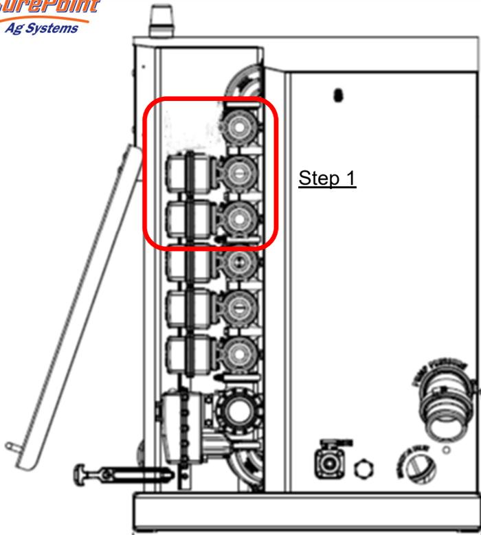
1. Remove mounting bolt, and top clamp and gasket in order to remove top 3-valve manifold, leaving 90° sweep elbow in place. Save clamps and gaskets for re-assembly.
