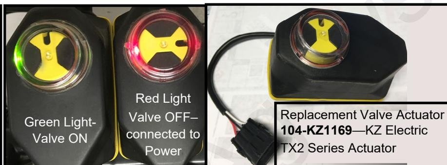
**This is a 3-way valve.** If product will not flow when valve is ON, either move the outlet hose to the other outlet port, or remove actuator and rotate valve ball 180°, and replace actuator. Product should flow
