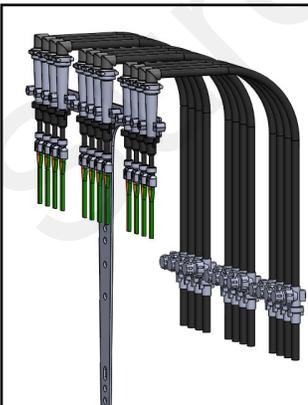
Mount flow indicators in banks (can be on one or multiple brackets). Dual metering tube Y's will attach to bottom of flow indicator. Top of flow indicator outputs through check valve to the row.
