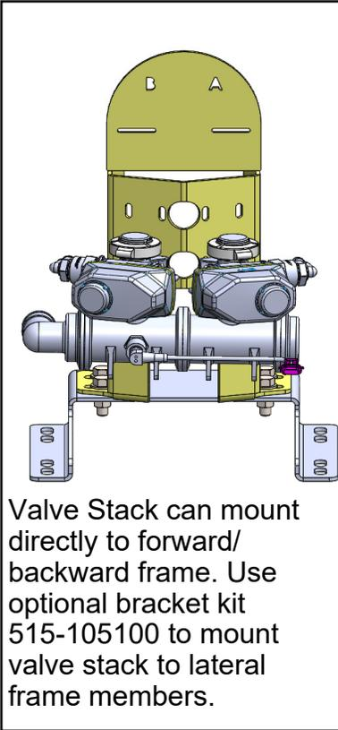
Feed into the section valve stack using 3/4", 1", or 1-1/2" hose from the pump. Each section valve output hose may be split using tees or crosses to feed the necessary number of banks per section.
