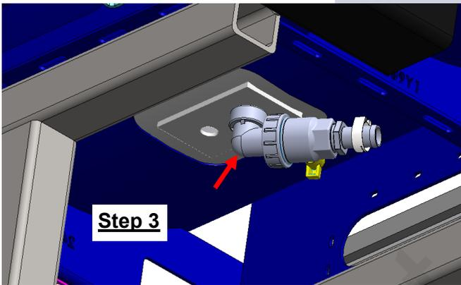
3. Attach the Manifold x Pipe Thread adapter fitting into the bottom of the 400 gallon tank and assemble tank fill valve assembly as shown (Reference Page 2)
