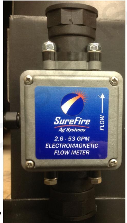
1. **Check for constant 12 V power on the harness that connects to the flowmeter.** (Need power and ground wire— **B & C (1&2)**— Constant 12-13 V-check with voltmeter) Should have 4-5 volts between Signal and Ground.
