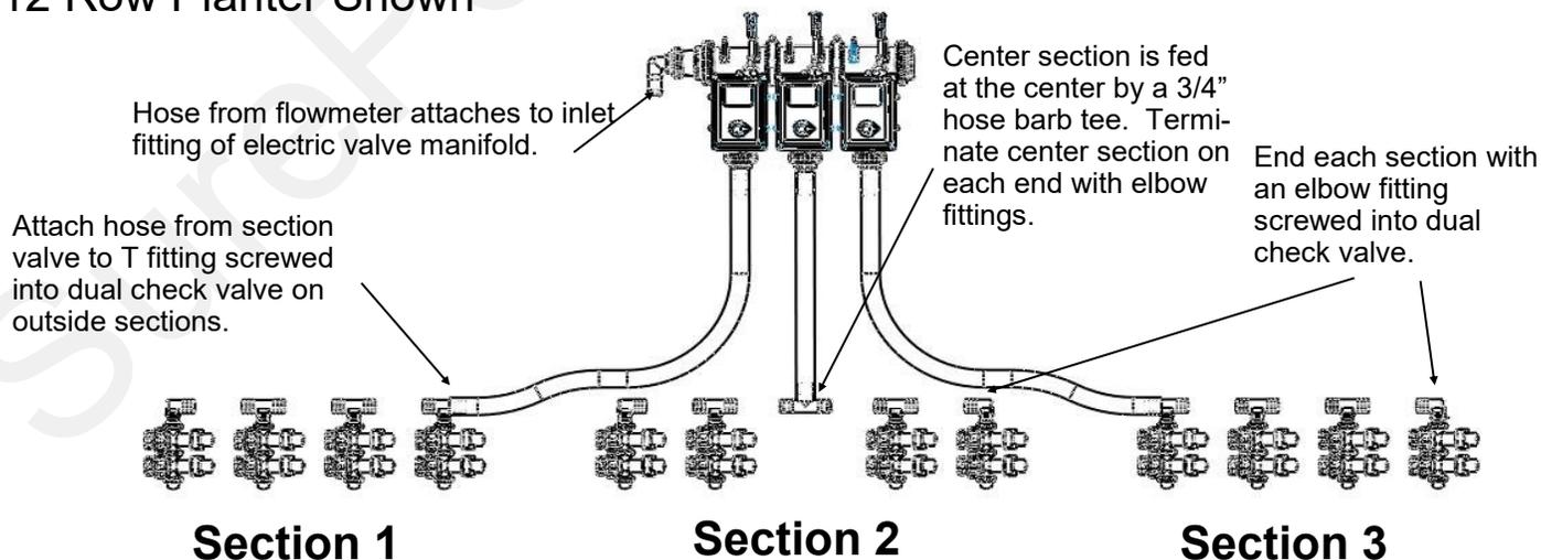
Hose from flowmeter attaches to inlet fitting of electric valve manifold.
