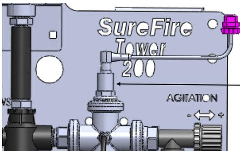
Pressure Sensor (3 wire type) with harness
