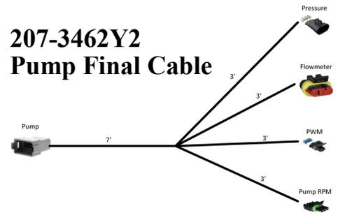
If the system only has 1 or 2 sections, use 207-3461 Y2 Final Harness and **Do Not** use section harness 207-3463Y1.
