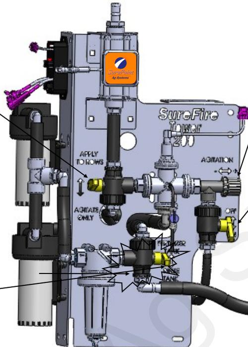
**Agitation Adjust Valve:** This valve adjusts how much flow returns to the tank while working in the field.
