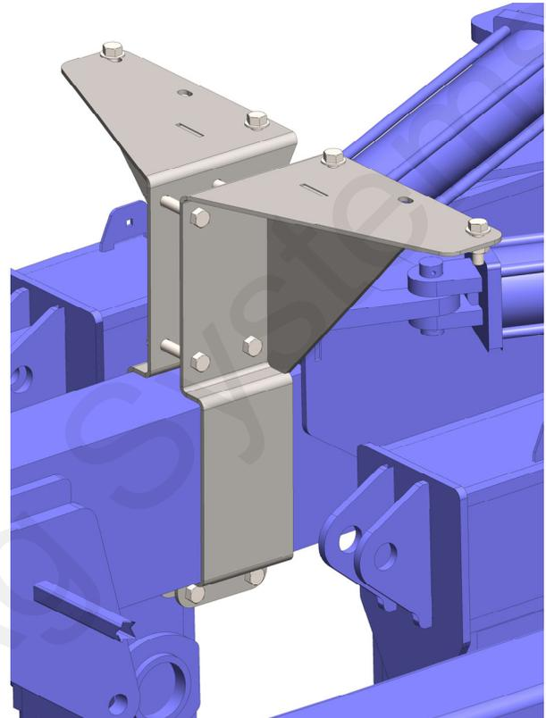
3. Set the cradle on the supports, adjusting the front support as necessary. Use 5/8" bolts to hold the cradle to the supports.
