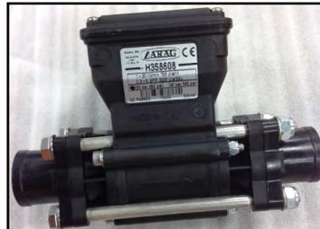
Serial number label on side also shows pulses per gallon.
