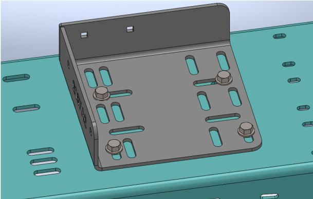
3. If section valves are not used, mount BOM 520-00-045000 (instruction sheet 396-2602Y1) as shown at right.
