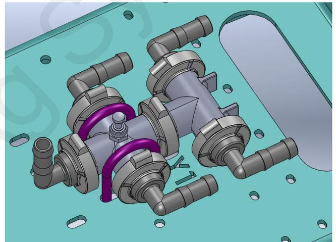
**Note:** Both the KZ and the Banjo section valves will fit underneath the hydraulic motor on the PumpRight pumps.
