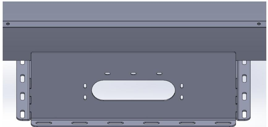
Bolt pump bracket through the slots on the side of the cradle.
