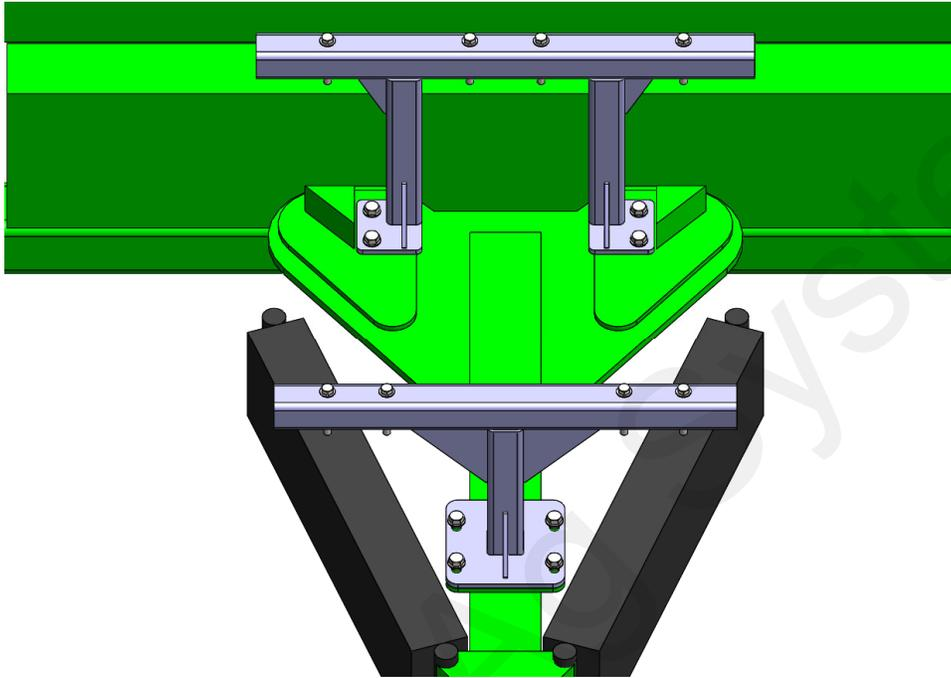
3. Set cradle on stands and bolt down using 5/8" bolts in locations shown above. Stands may be adjusted forward and backwards as necessary.
